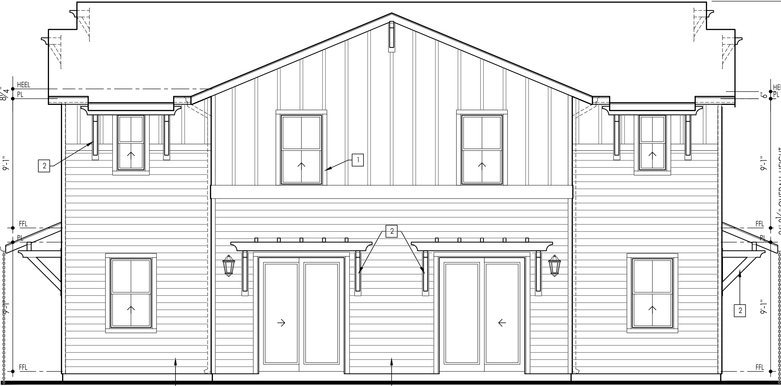
FARMHOUSE Front Elevation SCALE: 1/4"=1'-0" AT 22"X34" SCALE: 1/8"=1'-0" AT 11"X17"
