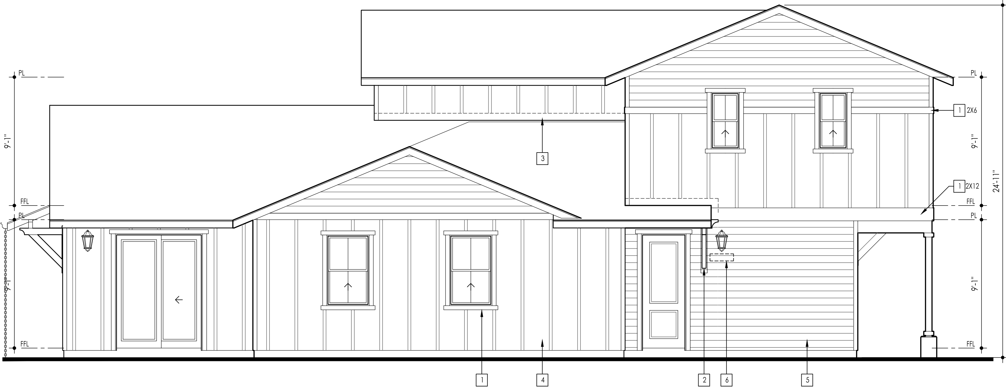
FARMHOUSE Front Elevation SCALE: 1/4"=1'-0" AT 22"X34" SCALE: 1/8"=1'-0" AT 11"X17"
