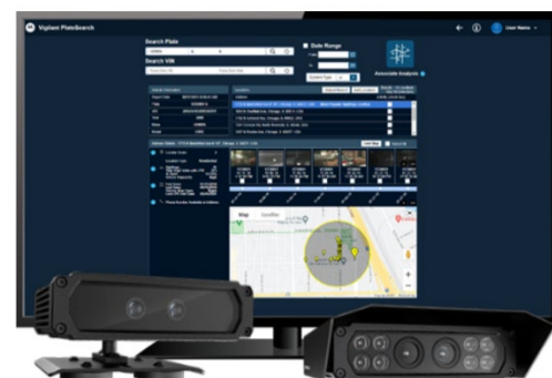
Example of vehicle mounted LPR cameras and dashboard
