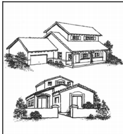
Figure 6-10a: Architectural design should facilitate the transition between stories
